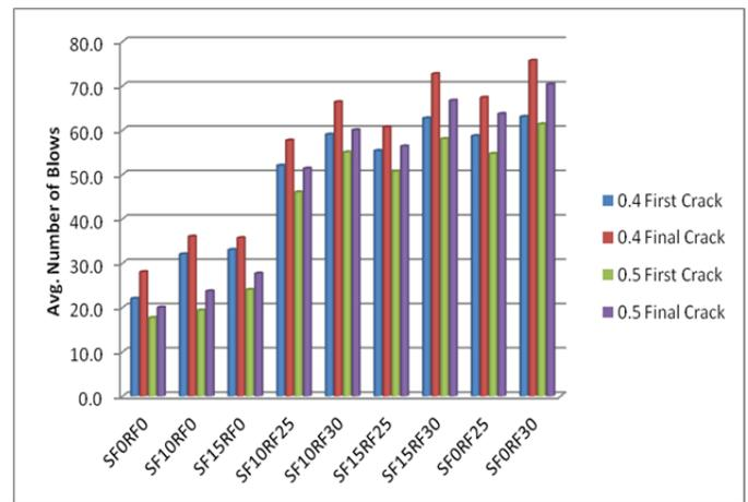
Fig. 5 Number of blows for Initial & Final crack
