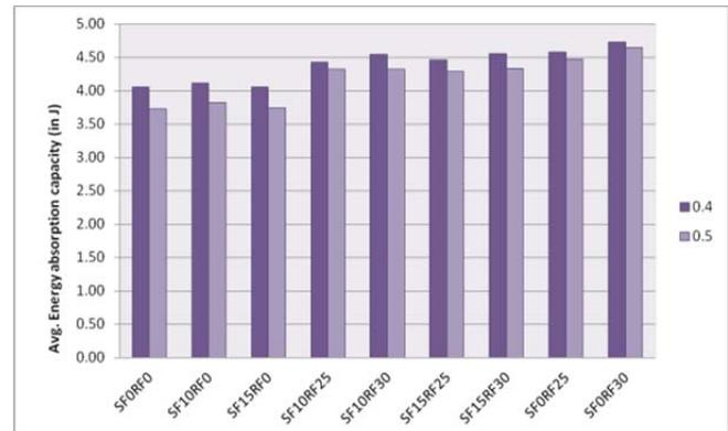
Fig. 8: Energy Absorption Capacity (Rebound Test)
