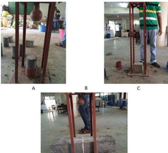
**Fig. 1: A. Impact Resistance Under Drop Weight Test , B. Impact Resistance Under Flexural Loading and C. Impact Resistance Under Rebound Test**
